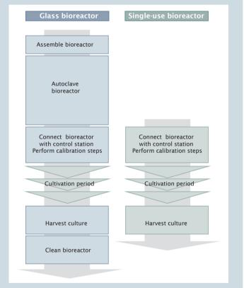
**Fig. 3:** Sequence of events in bioprocess runs using glass and single-use bioreactors.
