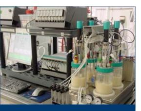
Figure 1. DASGIP system for biomass and protein optimisation and reaction engineering.
