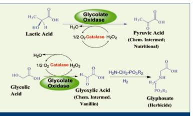
Figure 2. Glycolate oxidase (GO) now serves as a one enzyme one optimised process and several products platform. The process platform has been patented.
